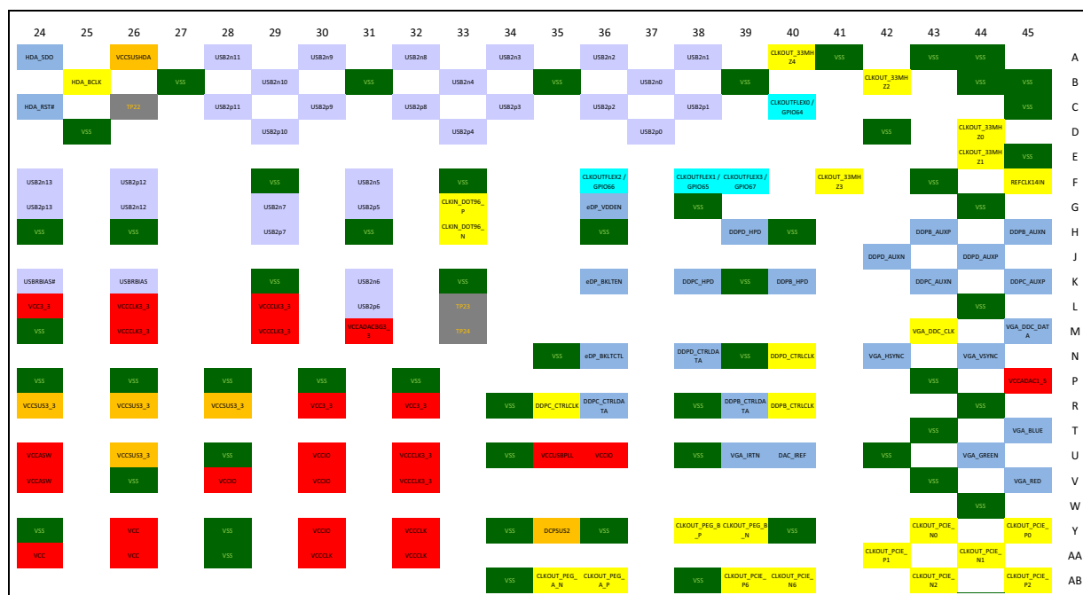
Figure 6-8. Mobile PCH Ballout (Top View - Lower Right)
